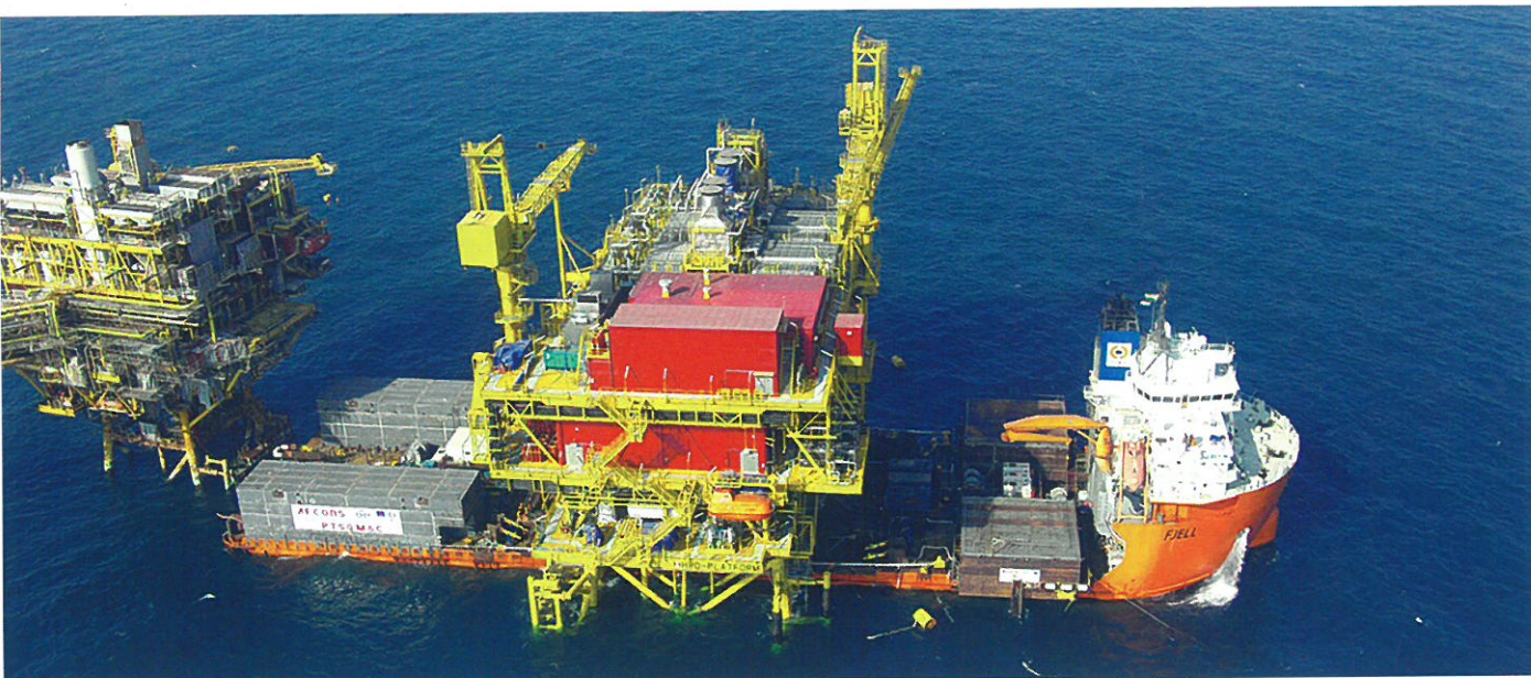
▲ The HRD Process Platform, Mumbai High, used float over methodology on Indian waters for the first time.
